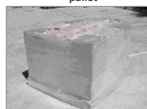
Figure 3 - Correctly wrapped pallet
